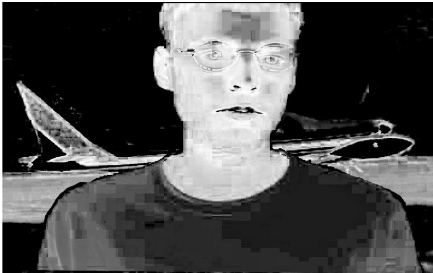
Figure 3.4: loglikelihood image (1-max. log likelihood value, the pixel with the value between 1 and maximum are scaled depending on its probability to be a skin pixel, the other pixels are set to zero)
